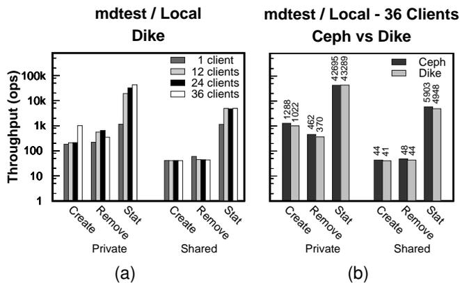
Fig. 12. Performance of mdtest file operations across different numbers of clients. We consider files distributed over private or shared folders of Dike (a) in comparison with the original Ceph (b). Dike uses 36 tenants to assign a separate tenant per client.
