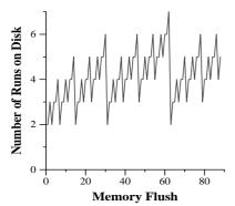
Figure 1: Several recent systems maintain the inverted file on disk across multiple partial indexes (runs) [6, 16]. When they retrieve the postings of a term, they need to access multiple runs of the inverted file. The x axis refers to the time instances at which memory contents are flushed to disk (Based on Wumpus with Hybrid Logarithmic Merge over the 426GB GOV2 [6].)
