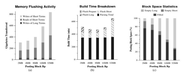
Figure 5: (a) As the size of the posting block increases, the system transfers more data between memory and disk during merging. (b) As the posting block becomes larger, there is a shift of the flush time from long terms to short. Setting  $B_p = 8MB$  strikes a good balance between the flush time of the different term types. (c) Empty space in posting blocks increases with their size, mostly due to dedicating separate blocks to each long term.
